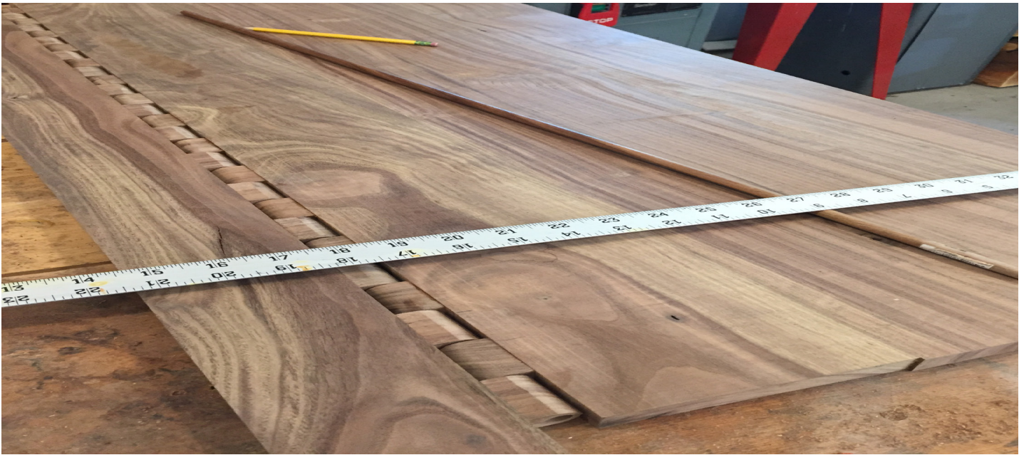
Metal-free hinge. A long hardwood dowel joins the pieces to create a strong and attractive integral piano hinge.
