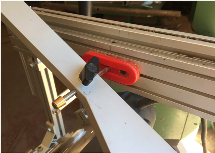
Holes first. On this project and many others, Murray relies on the PantoRouter for boring extremely precise holes and mortises. This is done by indexing the hole placement using the center hole in the templates. Once the first one is setup and stops are set, dozens more can be created in just a few minutes. Don's usual method is to bore the holes first, while the parts are square, and then shape them afterward.
