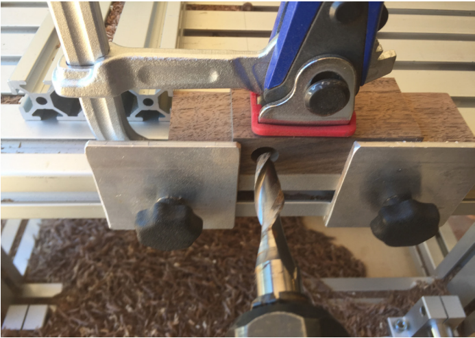
Holes first. On this project and many others, Murray relies on the PantoRouter for boring extremely precise holes and mortises. This is done by indexing the hole placement using the center hole in the templates. Once the first one is setup and stops are set, dozens more can be created in just a few minutes. Don's usual method is to bore the holes first, while the parts are square, and then shape them afterward.
