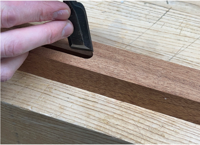
Use a wide chisel referenced off of the mortise wall to define the rectangular outline of the mortise.
