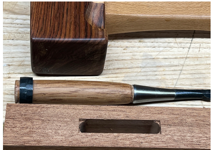
Using a mallet and a narrow chisel, follow the outline of the scribed marks. Since this is the show face, carefully remove about 1/8" deep of material without cutting past the line to establish a perfect outline of the through tenon.
