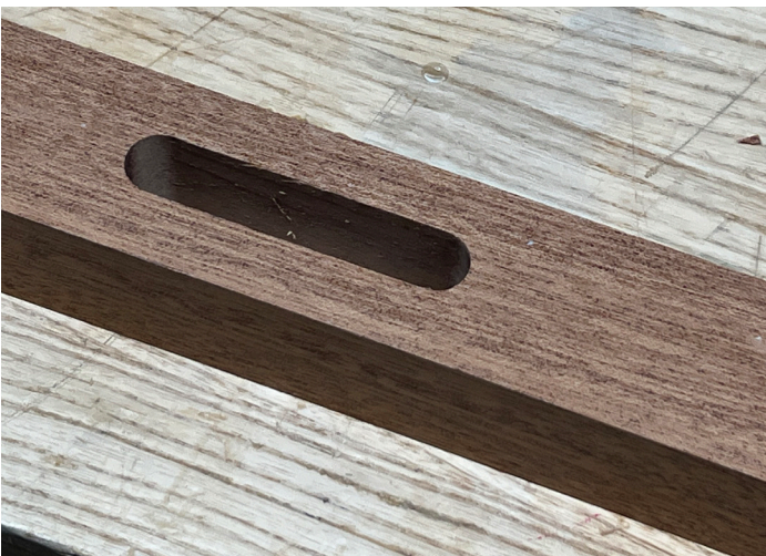
Flip the workpiece over so the back side of the mortise is up. Use a square to locate a narrow chisel where the mortise ends. This location is less critical because it will never be visible.
