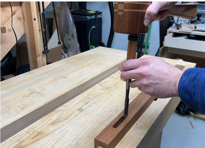
Using a mallet and a narrow chisel, follow the outline of the scribed marks. Since this is the show face, carefully remove about 1/8" deep of material without cutting past the line to establish a perfect outline of the through tenon.
