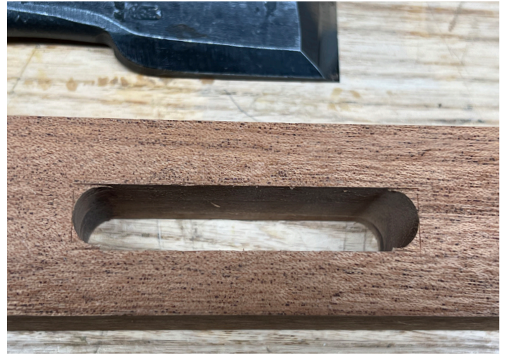
Use a wide chisel referenced off of the mortise wall to define the rectangular outline of the mortise.
